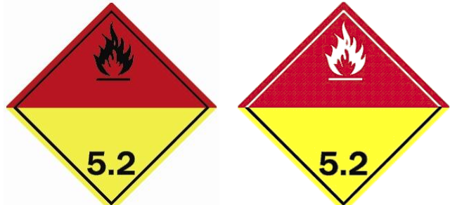
(Nr. 5.2) Symbol (flame): black or white; Background: upper half red; lower half yellow; Figure "5.2" in bottom corner
